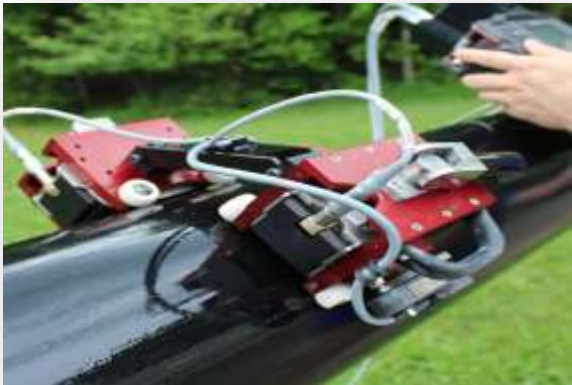
Medium Range Ultrasonic Test (MRUT)
